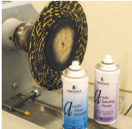
▲ Pic.20 Sanding, sealing and then lacquering is the best finish for coloured and textured work. The rub-on finish of acrylic sprays can move the colour around on the surface
